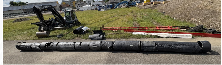
15 meters of 3D-printed pipe at Innovationspark Zürich
